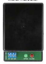
The MDM Actuator delivers up to 250 in/oz. (15.62 in/lbs.) of torque that powers the RTM open and closed. This powerful motor allows the damper to handle higher static pressures and can be modulated using the SPS or SPC Static Pressure Switch or similar type control.
