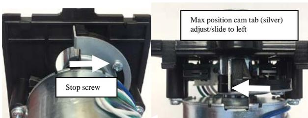
Move the adjustable cam (silver section of cam) to the left to adjust the maximum position. Make sure to re-tighten the cam locking screw and power. Reattach the actuator cover.
