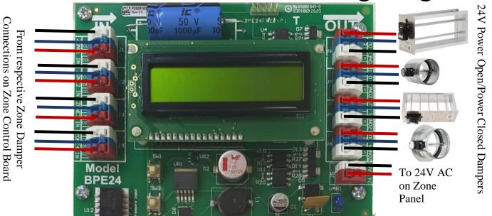
NOTE: If there is a Specific zone that should not be used to relieve air, wire zone damper directly to zone panel.
