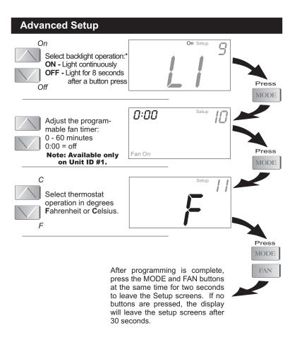
\*For increased battery life the backlight should be set to OFF unless the ACC0800 RF power supply adaptor is used to power the thermostat.
