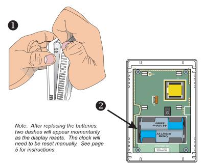
Important: To ensure proper operation use only AA LITHIUM batteries.
